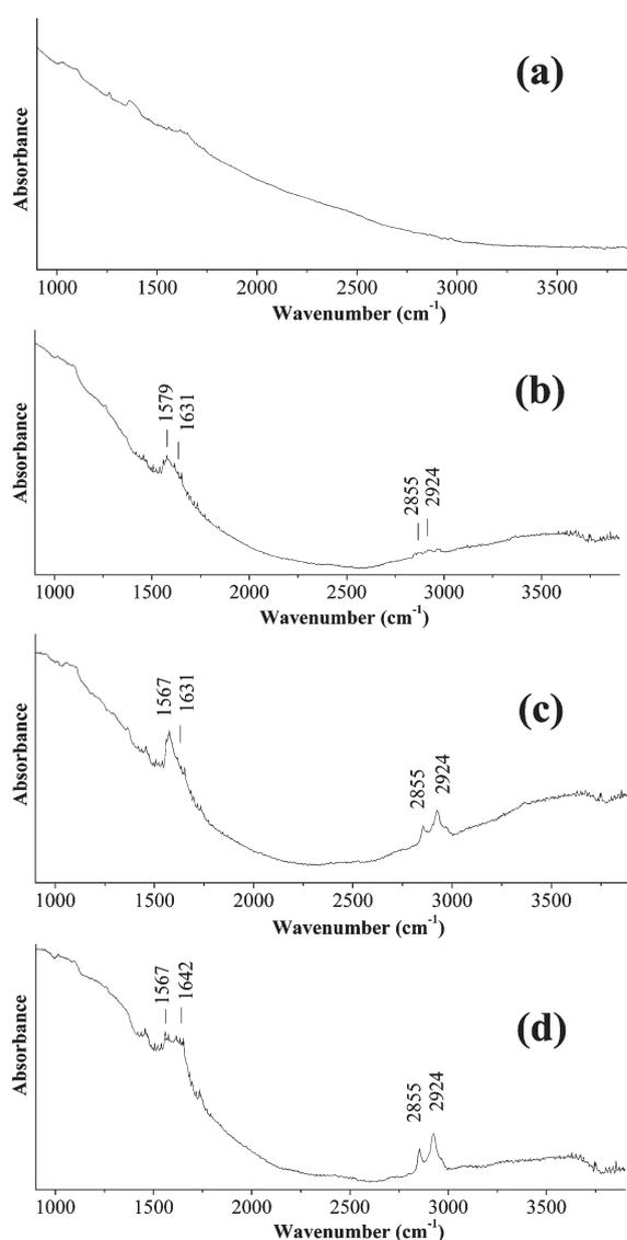
**Fig. 2** FTIR spectra (baseline uncorrected) of the oxidized SWNTs before and after their gas-phase treatment with 1,8-diaminooctane, L-alanine and  $\epsilon$ -caprolactam: (a) SWNT<sub>ox</sub>, (b) SWNT<sub>ox</sub>18, (c) SWNT<sub>ox</sub>18A, and (d) SWNT<sub>ox</sub>18C.
