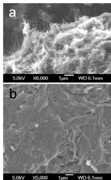
**Fig. 7** Comparison of SEM images of (a) SWNT<sub>ox</sub> and (b) SWNT<sub>ox</sub>18C samples.
