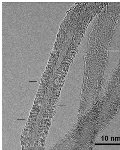
**Fig. 4** A typical TEM image of MWNT18C. The electron beam was focused on the center of the left nanotube, where segments of Nylon 6 chains are marked with black bars. The white bar points to the section where the beam focuses on the front or rear nanotube surface wrapped with polymeric chains.
