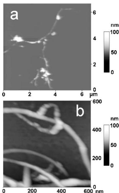
**Fig. 8** AFM images of (a) SWNT<sub>ox</sub>18C and (b) MWNT18C samples, deposited onto mica supports from isopropanol.
