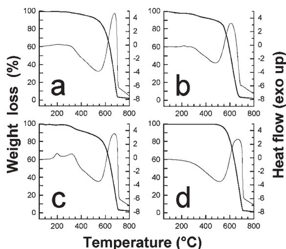
**Fig. 9** TGA (thick lines, left axis) and DSC curves (thin lines, right axis) of the nanotube samples: (a) MWNT18, (b) MWNT18A, (c) MWNT18C, and (d) MWNTC.
