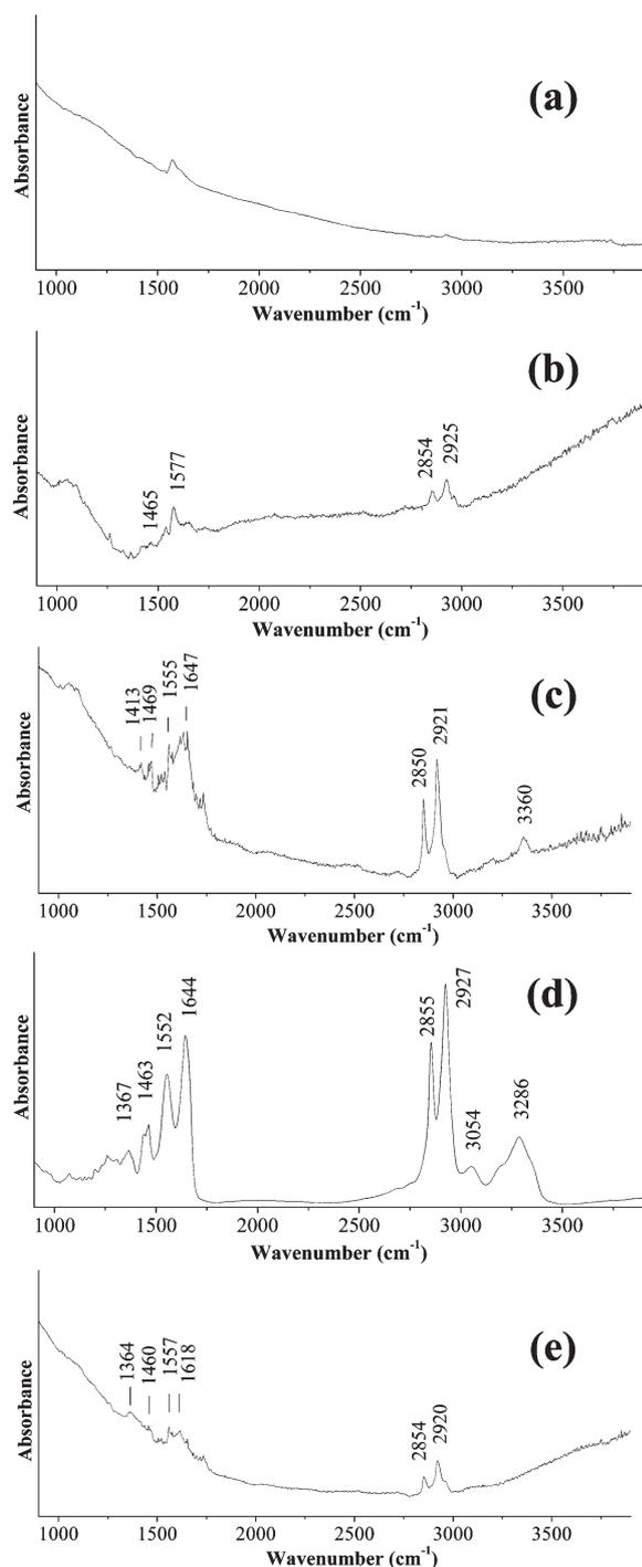
**Fig. 3** FTIR spectra (baseline uncorrected) of the pristine MWNTs before and after their gas-phase treatment with 1,8-diaminooctane, L-alanine and  $\epsilon$ -caprolactam: (a) MWNT, (b) MWNT18, (c) MWNT18A, (d) MWNT18C, and (e) MWNTC.
