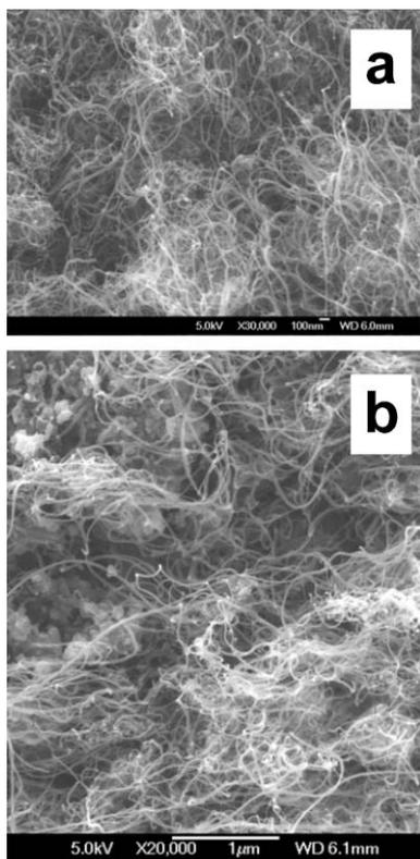
**Fig. 5** Comparison of SEM images of (a) pristine MWNT and (b) MWNT18C samples.
