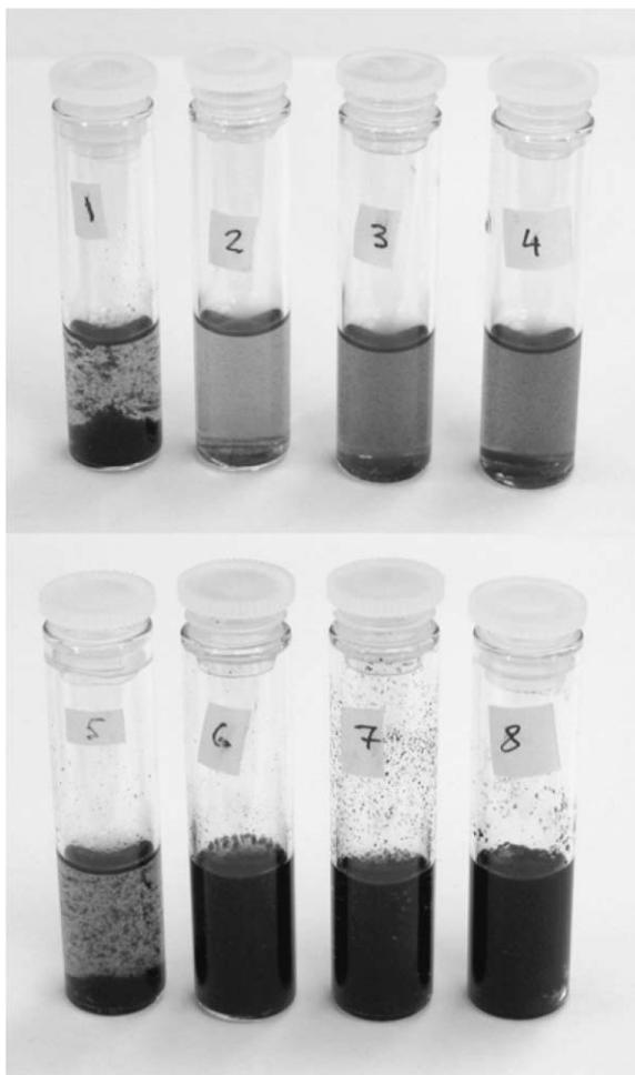
**Fig. 1** Dispersions of the different nanotube samples 15 min after 5 min of ultrasonication in isopropanol: (1) SWNT<sub>ox</sub>, (2) SWNT<sub>ox</sub>18, (3) SWNT<sub>ox</sub>18A, (4) SWNT<sub>ox</sub>18C, (5) MWNT, (6) MWNT18, (7) MWNT18A, and (8) MWNT18C.
