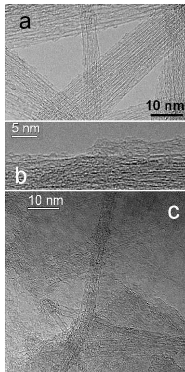
**Fig. 6** Comparison of TEM images of (a) SWNT<sub>ox</sub> and (b,c) SWNT<sub>ox</sub>18C samples: (b) amorphous material on the surface of SWNT<sub>ox</sub>18C bundle; (c) the nanotubes dispersed in the polymer phase.
