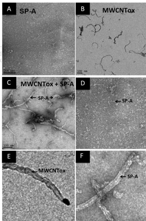
**Fig. 4.** Transmission electron micrographs show the binding of SP-A to MWCNT<sub>ox</sub>. (A) SP-A alone, (B) MWCNT<sub>ox</sub>, (C) MWCNT<sub>ox</sub> + SP-A. The acid treatment greatly reduces the size of MWCNTs. The average size of shortened MWCNT<sub>ox</sub> is between 300 nm and 1 μm. The walls of MWCNT<sub>ox</sub> are completely coated with SP-A as indicated by black arrows. (E)–(F) shows a magnified view of (A)–(C).
