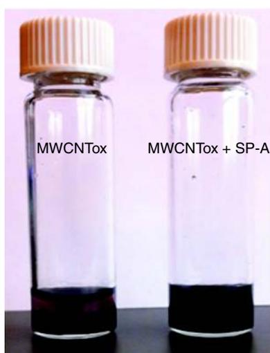
**Fig. 2.** Dispersibility test of acid-treated MWCNTs in Opti-MEM. Acid-treated carbon nanotubes (MWCNT<sub>ox</sub>, left side) and MWCNT<sub>ox</sub> coated with SP-A (MWCNT<sub>ox</sub> + SP-A, right side) suspended in Opti-MEM (without added serum) for 1 h after five min of sonication.
